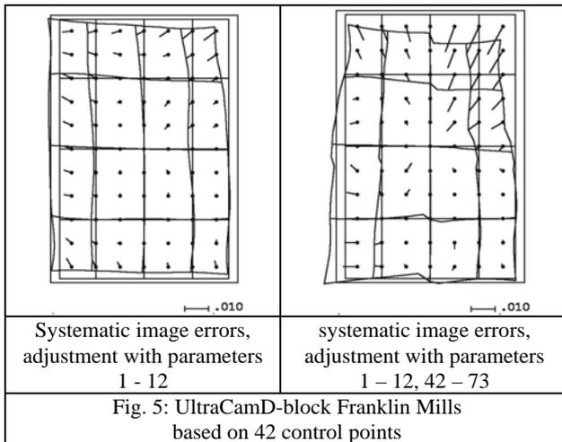
The adjustment of the UltraCamD-block with self calibration is slightly improving the results at independent check points. Also the UltraCamX-images have not negligible systematic image errors (fig. 6). The size is on the level of the UltraCamD (fig. 5) and approximately twice like for the DMC-images (fig. 4).
