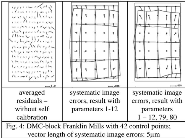
Also block adjustments with 15 and 8 control points have been made. The not used control points have been handled as independent check points. Only the adjustment with 8 control points showed a small improvement of the Z-component by adjustment with self calibration. Of course the test block has a limited size, so the systematic image errors cannot sum up and deform the block.
