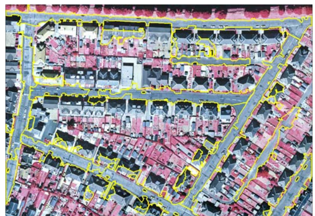
Figure 4. Road parts extracted in subset 2 (yellow).
