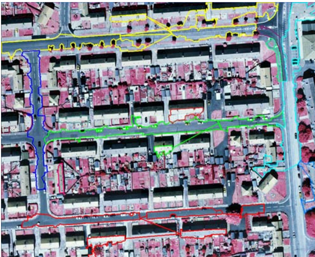
Figure 6. Road subgraphs (without DSM) for subset 1. Different colours represent different road subgraphs.
