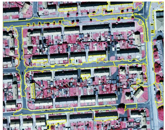
Figure 3. Road parts extracted in subset 1 (yellow).
