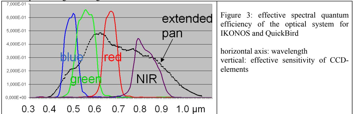
Figure 3: effective spectral quantum efficiency of the optical system for IKONOS and QuickBird
