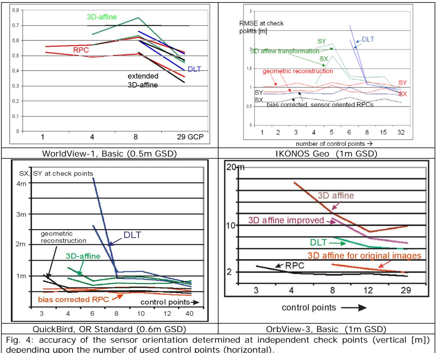
Fig. 4: accuracy of the sensor orientation determined at independent check points (vertical [m]) depending upon the number of used control points (horizontal).
