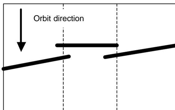
Figure 2: horizontal location of CCD-line-sensors in the image plane
