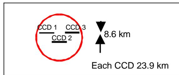
figure 1: separation of the 3 CCD-sensors in the PAN-camera
