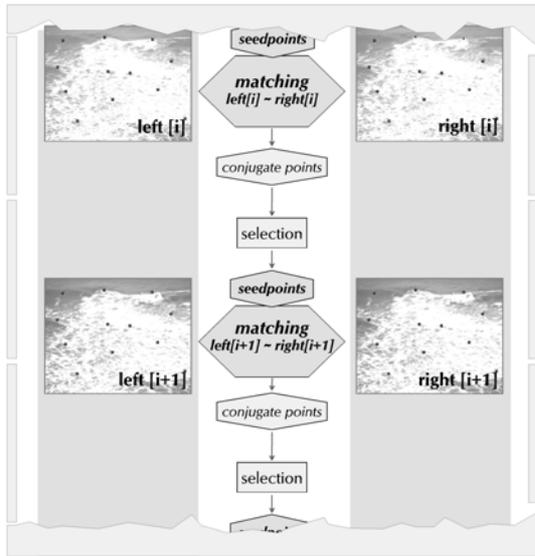
Figure 3. Principle of transfer of seed points
