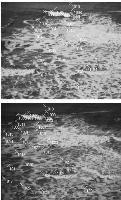
Figure 5. Measured seed points (above: left image, below: right image)
