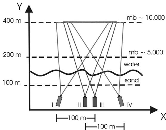
Figure 2. Camera constellation in planimetry
