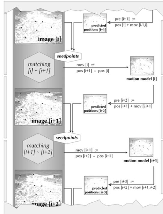
Figure 4. Principle of motion models
