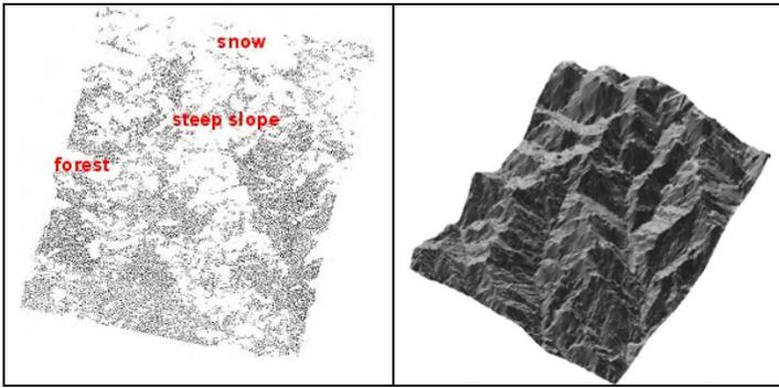
Figure 9. results of image matching with IRS-1C in the Himalayas, left: matched points, right: 3D-view of the generated DEM
