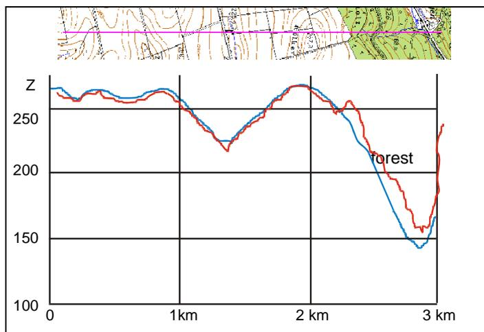
Figure 16. height profile through a DEM generated by SRTM-X-band and a corresponding DEM of the survey administration – upper part: topographic map
