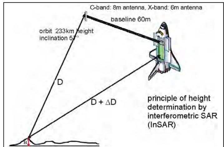
Figure 16. principle of INSAR during the SRTM-mission
