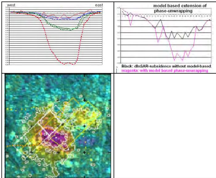
Figure 18. subsidence in coal mining area determined by DINSAR (Spreckels et al 2001)
