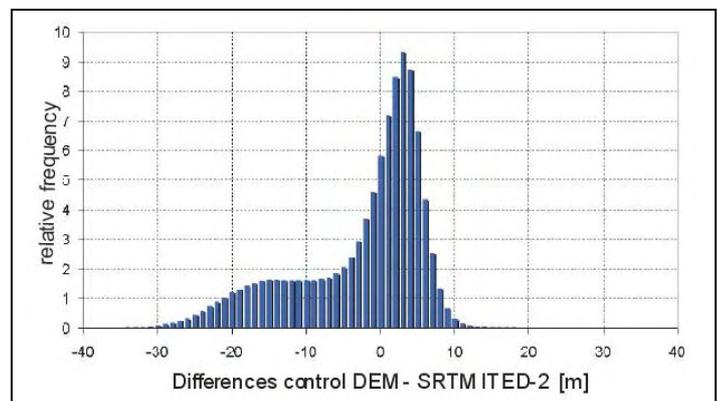
Figure 15. frequency distribution of the discrepancies in a SRTM X-band DEM
