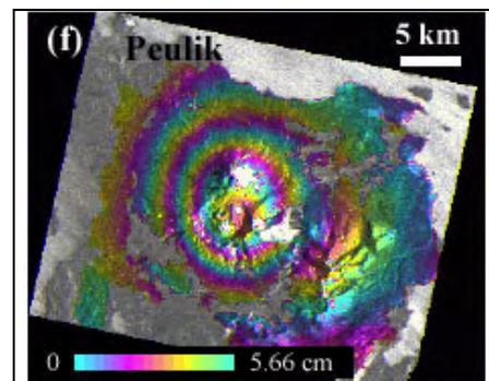
Figure 17. height changes of a volcano (Zhong et al 2002) determined by DINSAR based on ERS 1 and ERS 2
