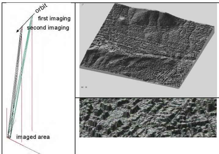
Figure 12. left: configuration of IKONOS stereo model right: generated DEM – lower part: detail in city area showing buildings in the DEM
