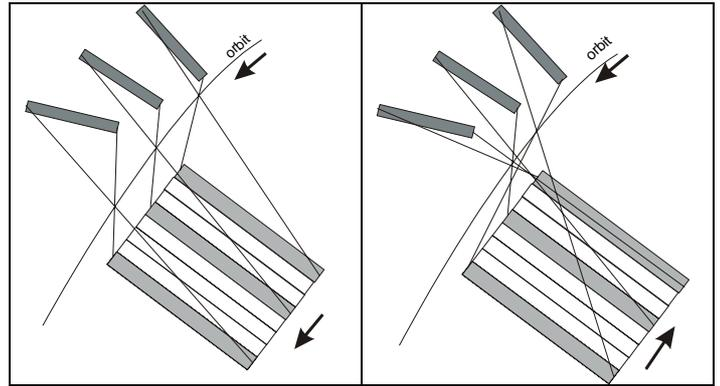
Figure 5. principle of imaging – sensors with flexible view direction
