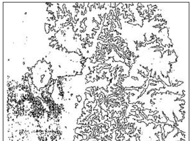
Figure 20. contour lines of a DEM determined by automatic matching of MOMS-images
