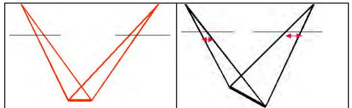
Figure 7. left: normal case, horizontal ground right: inclined ground – different size in image
