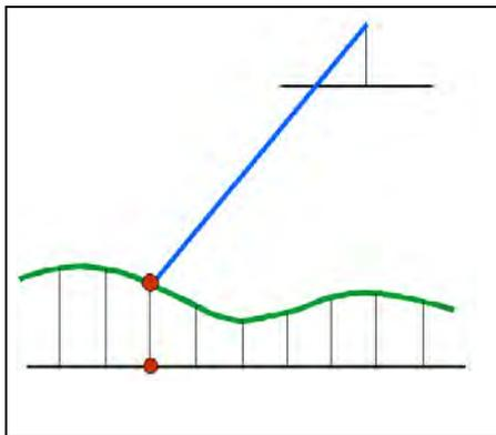
Figure 2. correct geo-location by means of 1 image and a DEM (orthoimage)
