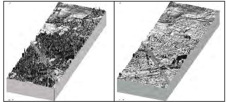
Figure 19. left: original DSM right: DSM filtered by program RASCOR to a DEM
