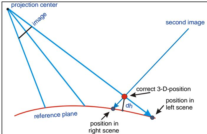
Figure 6. geometric relation between IKONOS Geo-images and the three-dimensional location of the imaged points
