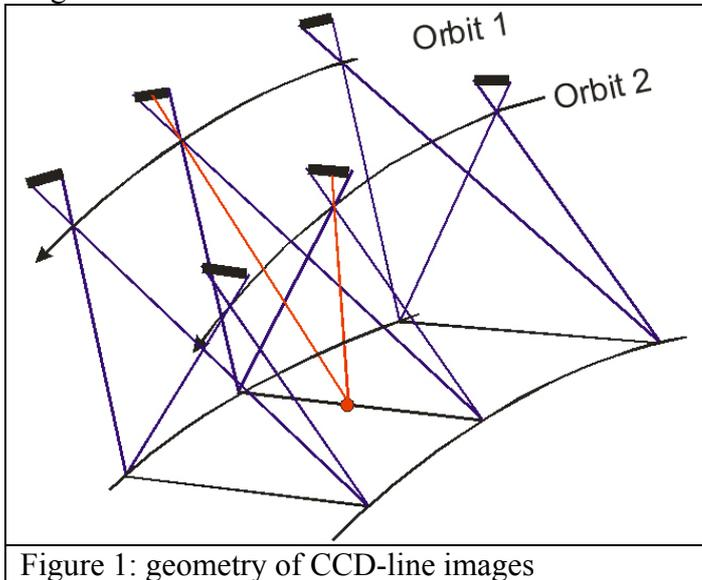
Figure 1: geometry of CCD-line images
