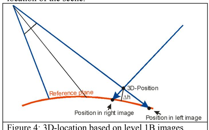
Figure 4: 3D-location based on level 1B images
