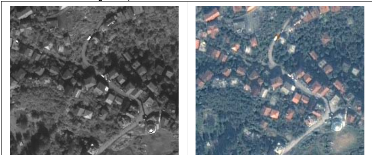
Fig. 8: influence of color to object identification left: panchromatic IKONOS right: pan sharpened IKONOS
