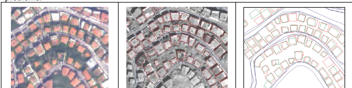
Fig. 10: mapping buildings left: QuickBird 2.4m GSD, center: pan 2.4m GSD, right: overlay
