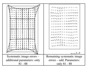
Figure 5: systematic and remaining systematic image errors UltraCam Eagle only with additional parameters 81 - 88
