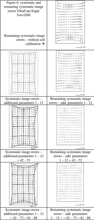
The UltraCam Eagle is fusing the 9 panchromatic sub-images of the 4 sub-cameras together. With the so called "monolithic stitching" (Ladstädter et al. 2010) the panchromatic sub-images are fitted to the green image which is based on one CCD-array with approximately linear three times lower resolution. This stitching improved the image geometry clearly against the former merging of sub-images; nevertheless the special additional parameters for the sub-images (parameters 32-73) have to be checked.
