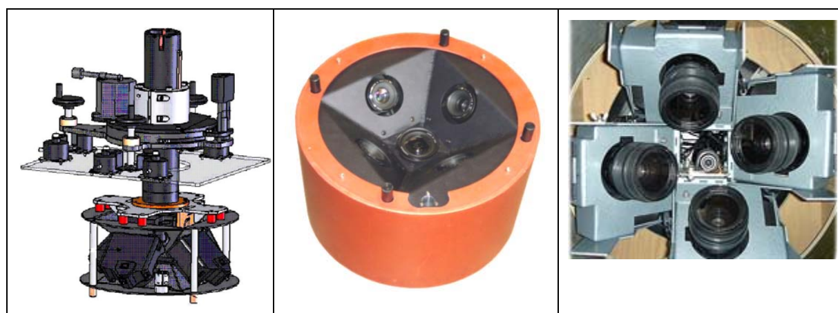
Figure 3. Track'Air MIDAS camera system – combination of 5 Canon EOS cameras
