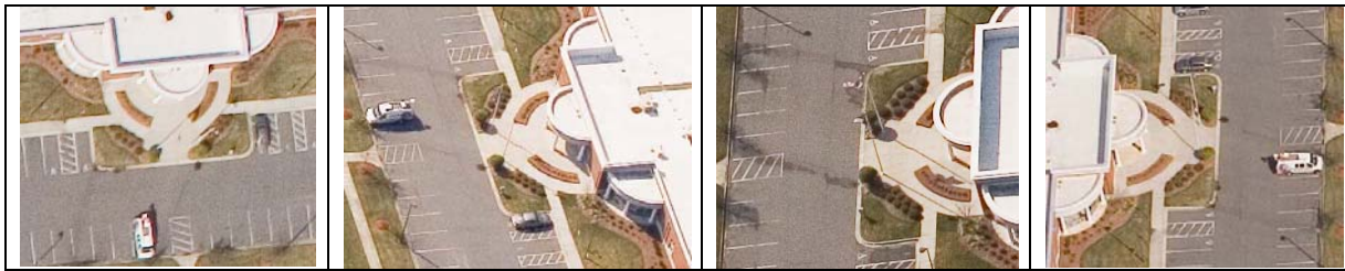
Figure 10. MultiVision image combination – images taken from different flight lines may cause differences of movable objects, vertical images (left) with smaller scale
