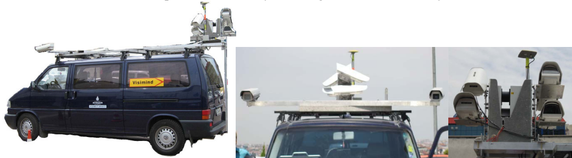
Figure 4. Sensor configuration on the mobile mapping van of VISIMIND AB
