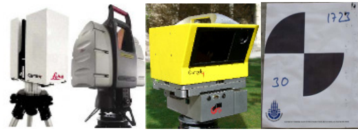
Figure 1. Terrestrial laser scanners used: Leica HDS4500, Leica HDS3000, and Optech ILRIS-3D, target for registration and geo-referencing of scans
