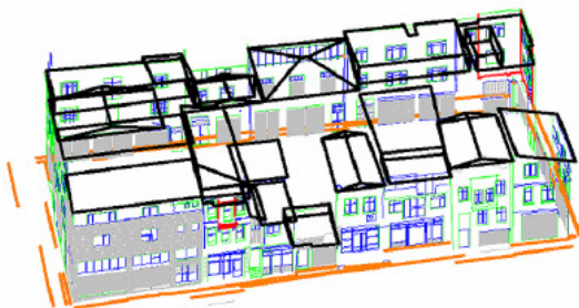
Figure 14. Combination of data from two different sources: 3D polylines of roofs based on aerial images and 3D polylines of facades from terrestrial laser scanning data
