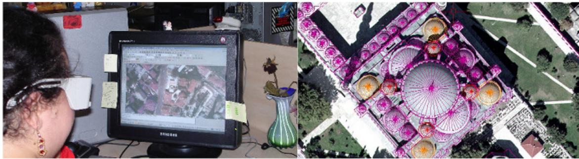
Figure 13. 3D mapping of roofs using Menci-software Z-MAP Foto in stereo mode
