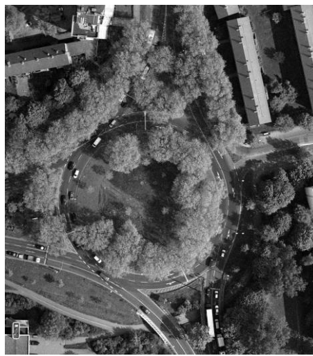
Figure 4-28: Illustrating an example in which the central island cannot be extracted due to heavy occlusions caused by trees and their shadows.
