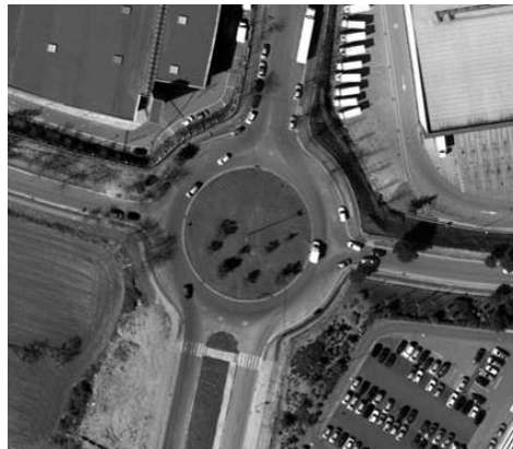
Figure 4-2: An example where our approach fails to extract the road arm due to a wide divider that exists within the roads in the bottom.
