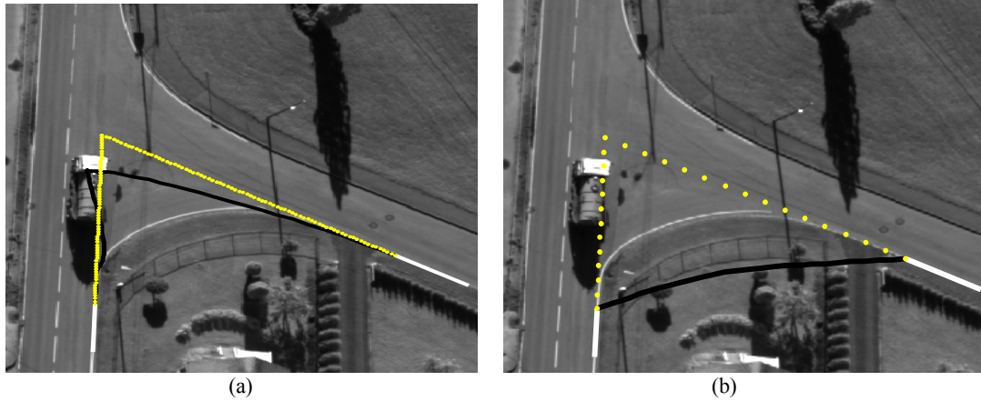
Figure 3-21 : Illustrating the snake behaviour with two different snake spacing values. (a) Snake spacing is 3 pixels, which signifies dense initial vertices (yellow), and the convergence threshold is 1/200 pixel. Here, the snake is caught by the truck and its shadow (black line). (b) Snake spacing is 15 pixels with the same convergence threshold. The optimized active contour cannot delineate the junction border even if the balloon force is active.
