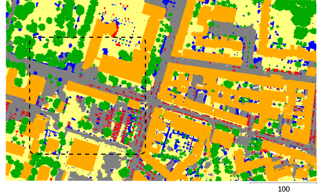
Figure 3. Result of the last CRF^P classification for the test area. The colors correspond to the classes road (grey), natural soil (yellow), low vegetation (blue), tree (green), building (orange), and car (red). The dashed rectangle illustrates the location of Fig. 4
