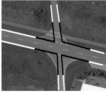
Figure 7. Illustration of the global initialization. Black lines are defined by two close endpoints and the intersection point of their respective road sides.
