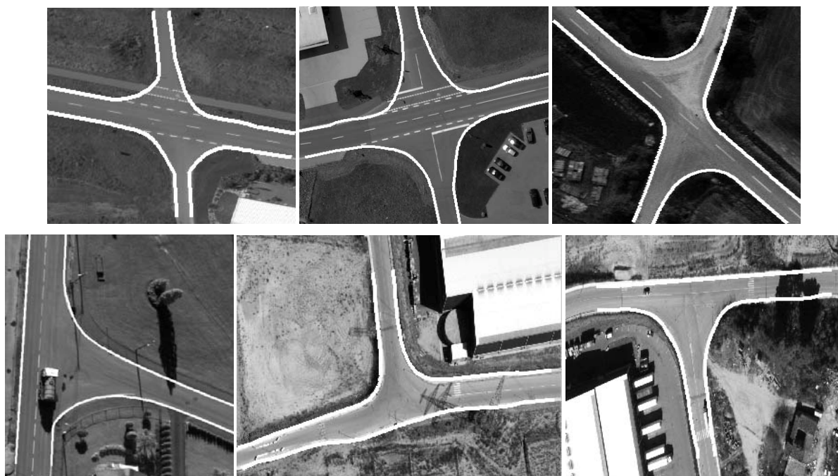
Figure 11. Top row image samples show rural areas and those in the bottom row are from suburb areas. In both groups, disturbances caused by road markings are resolved. Furthermore, the results in suburb areas are accurate even in the presence of shadows.
