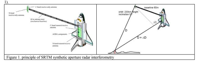
The C-band and X-band radar equipment was supported for the orientation by star tracker, gyros and GPS. Because of some mast vibrations, the accuracy of the orientation based on GPS, gyros and star trackers was limited,
