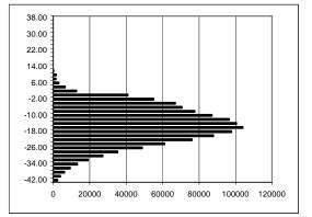
**Figure 8.** difference SRTM height model – reference DEM
