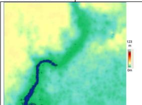
**16.** SRTM 1"-DEM of test Philadelphia filtered for elements not belonging to bare ground
