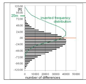
**Figure 5.** Frequency distribution of height differences between reference DEM and SRTM-DEM
