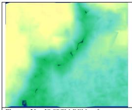
**Figure 20.** 3"-SRTM-DEM of test area Philadelphia, filtered for elements not belonging to bare ground
