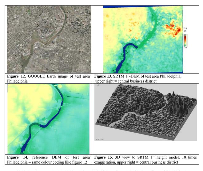
As obvious in comparing the SRTM height model with the reference DEM (figures 13 and 14) and also shown as 3D-view to the differential height model (figure 15), the SRTM height model is a DSM including an average of the
