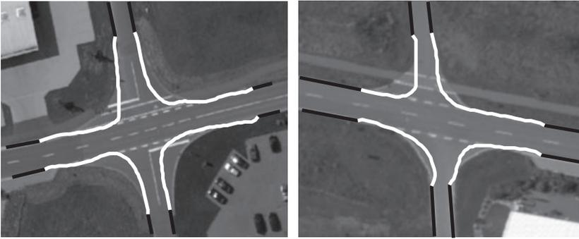
FIG. 8. Ziplock snake optimisation using a traditional force field as an external force. White curves are the result of snake optimisation. Black lines are the extracted road arms. Since the capture range of the external force field is small, the iterations are stopped near the initial positions.
