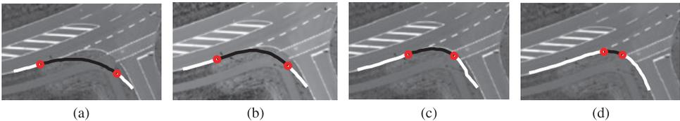
FIG. 11. The effect of the balloon force in four successive steps. In (a), the balloon force is applied for the first time. In (c), a slight deformation of the bottom-right active part close to the passive part can be observed and in (d) both active and passive parts captured the junction boundary correctly.
