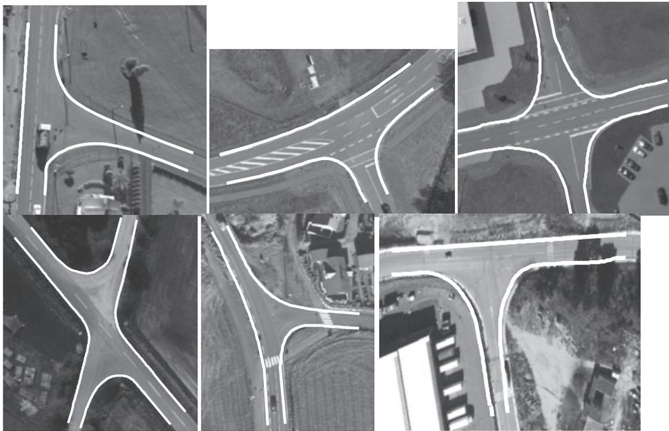
FIG. 15. Road junction extraction results. Image samples represent scenes that contain varying degrees of complexity including disturbances.
