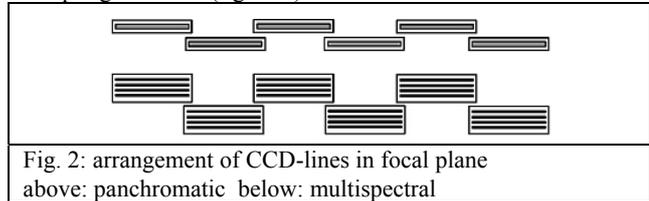
Fig. 2: arrangement of CCD-lines in focal plane above: panchromatic below: multispectral
