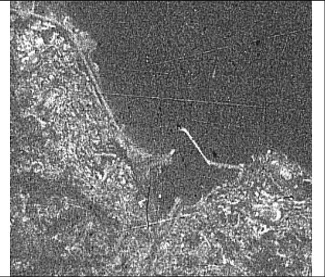
Fig. 6: scratches and film grain of a TK350 photo
