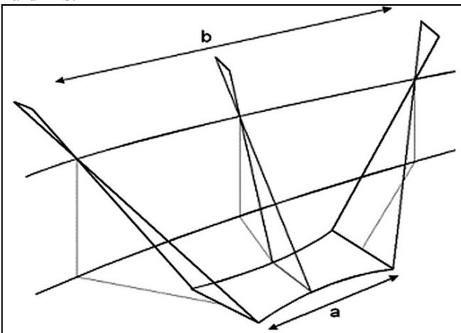
Fig. 1: enlargement of integration time with factor  $b/a$  by continuous change of view direction
