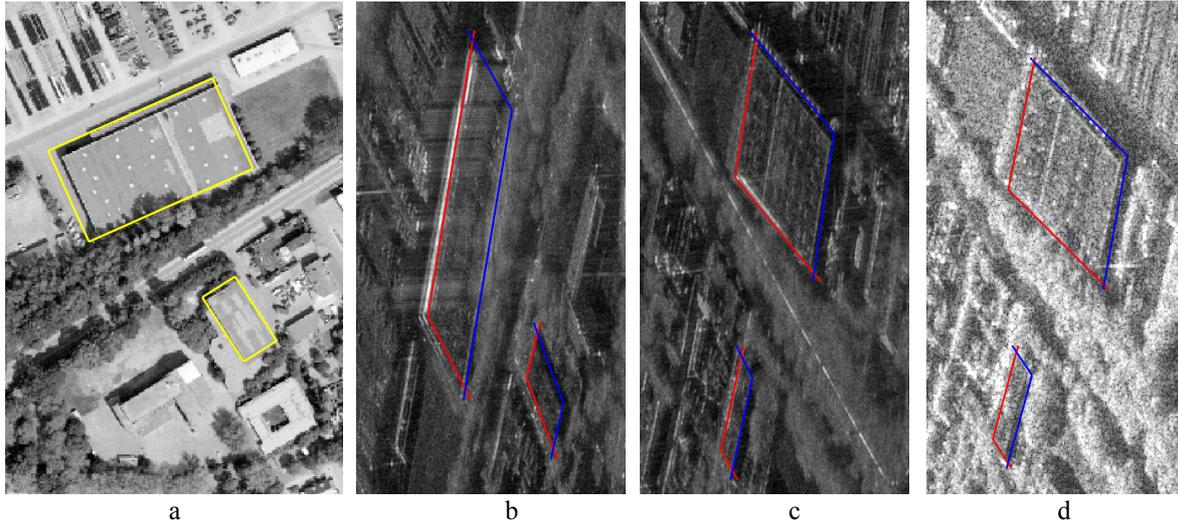
**Figure 2** Orthophoto overlaid by results of the building reconstruction (a), magnitude images overlaid by re-projected building footprints of D1 (b), D2 (c) and D3 (d); sensor close (red) and sensor far (blue) footprint lines
