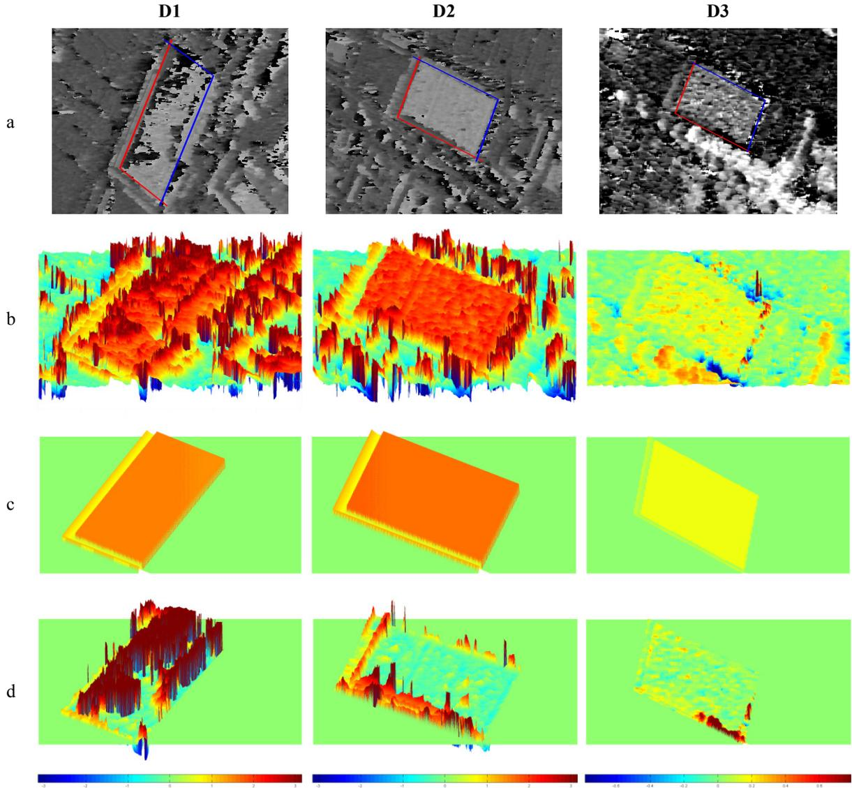
**Figure 3** Interferometric heights in slant range overlaid with re-projected building footprint (a), 3D visualization of real interferometric phases (b), of simulated phases (c), and differences between real and simulated phases
