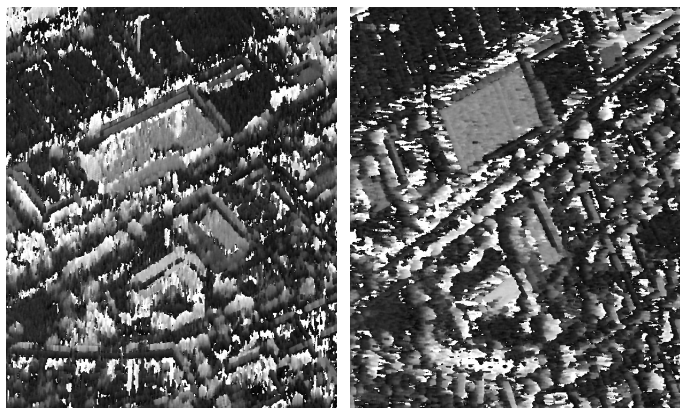
Figure 3. Part of interferometric height images of flight direction 1 (left) and direction 2 (right) in slant range geometry
