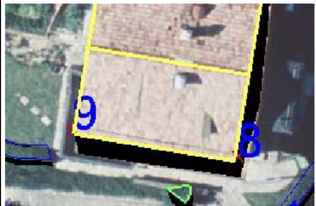
Figure 10: orthoimage with the corrected location of the building roof
