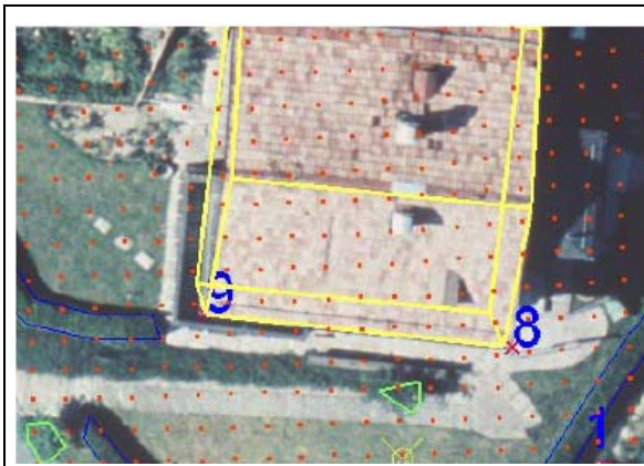
Figure 9: location of a building in a usual orthoimage based on a DEM including the bare ground
