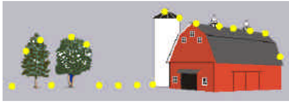
Figure 2: DSM - Yellow points belonging to surface of objects.
