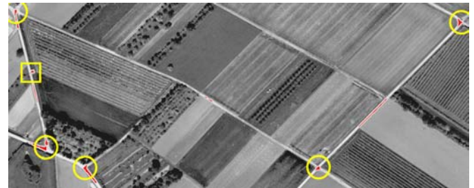
Fig. 6. Correctly recognized road junctions (marked with circles) and a position with a widening road (marked with square)
