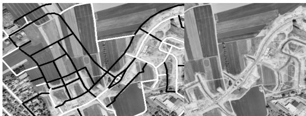
Figure 5. verification result for an updating situation due to road construction (ATKIS is up-to-date but not the imagery)
