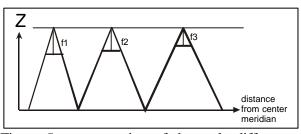
Figure 5: compensation of the scale difference between Z and X,Y by modified focal length
