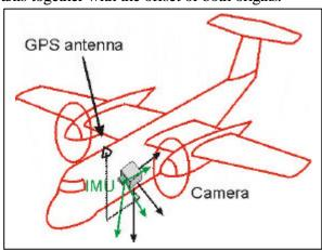
Figure 1: relation camera – IMU – GPS antenna
