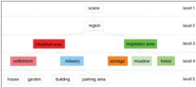
Figure 3: Semantic net for description of structural dependencies with respect to the verification of the area ATKIS objects in level 3 and 4.
