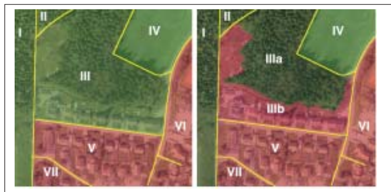
Figure 4: Typical analysis with regard to settlement and vegetation areas; left: expected ATKIS objects (numbered), right: the result of the automatic analysis.
