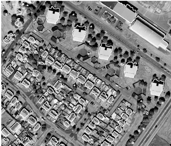
Fig. 4: Detected *BuildingAreas* with additional incorrectly assigned regions
