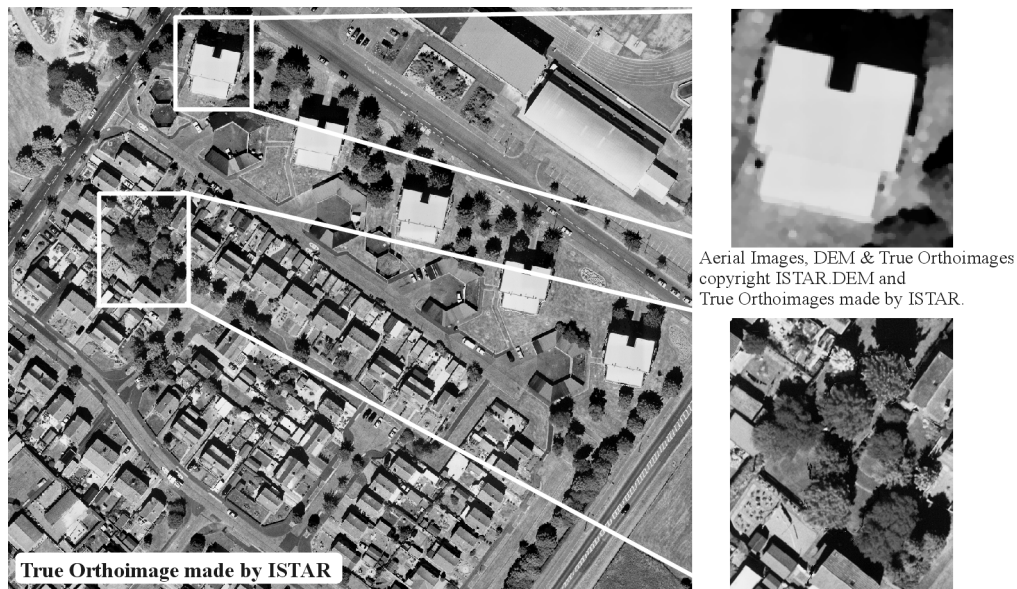
Figure 8: Overview of the test site “Grangemouth”, two enlarged subsets showing a building and trees in the orthoimage
