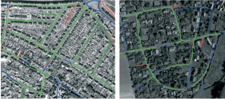
FIG. 3. Extracted road networks for the case when a DSM was used. Left: Grangemouth, with DSM. Right: Vaihingen, with DSM. True positives in green, false positives in red, false negatives in blue.
