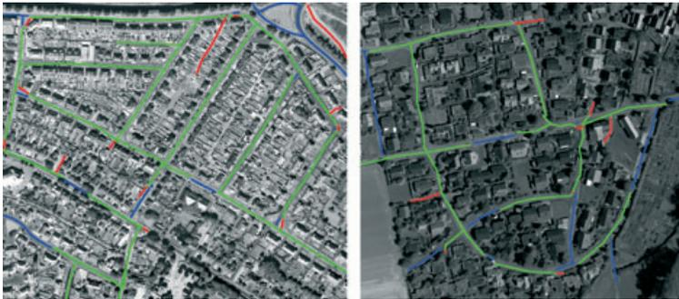
FIG. 4. Extracted road networks compared to reference without tree-covered roads. Left: Grangemouth. Right: Vaihingen. True positives in green, false positives in red, false negatives in blue.
