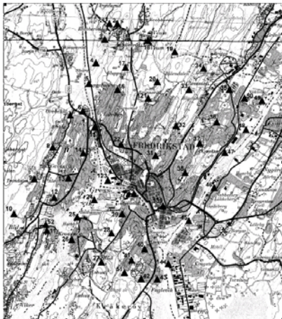
Figure 1: Test field Fredrikstad, the black triangles indicate the position of the ground control points
