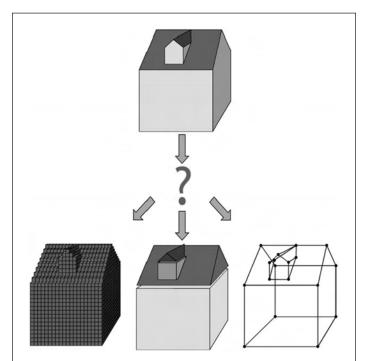
Figure 2. Three possibilities for 3D data structures of buildings: voxels (left), constructive solid geometry (center), boundary representation (right); from Pfund (2002).
