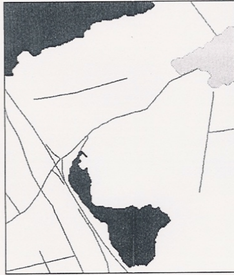
FIG. 8. Global context areas and roads extracted without modelling trees, showing forest (dark grey), settlement (light grey), open landscape (white) and roads (grey lines).
