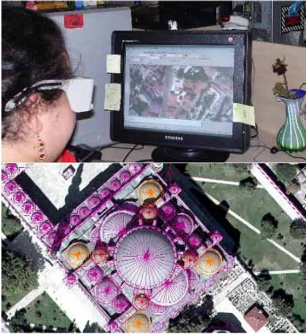
Figure 13. 3D mapping of roofs using Menci-software Z-MAP Foto in stereo mode
