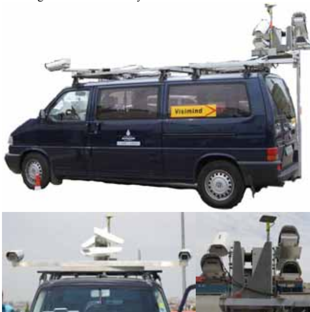
Figure 4. Sensor configuration on the mobile mapping van of VISIMIND AB
