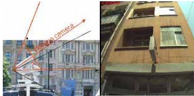
Figure 8. Oblique and horizontal camera integration in the mobile system (left), image taken by oblique camera (right)
