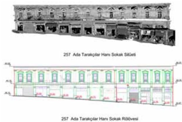
Figure 11. Part of the final product from façade mapping using terrestrial laser scanning data and photogrammetric images
