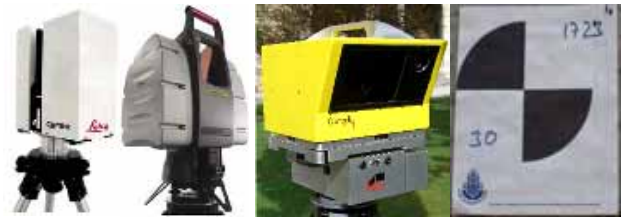
Figure 2. Used terrestrial laser scanner: Leica HDS4500, Leica HDS3000, and Optech ILRIS-3D, target for registration and geo-referencing of scans
