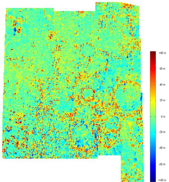
Figure 7. Results of bundle block adjustment (height diff.)
