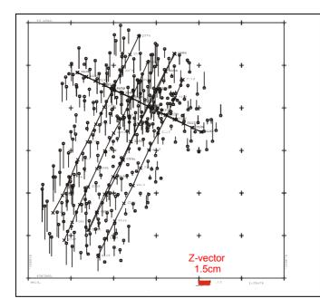
**Figure 5:** remaining Z-discrepancies of a combined intersection in the UTM-system with image coordinates improved by earth curvature correction and a unique change of the focal length by the mean scale of the UTM-system in the block
