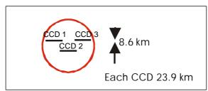
**Fig.1**: separation of the 3 CCD-sensors in the PAN-camera
