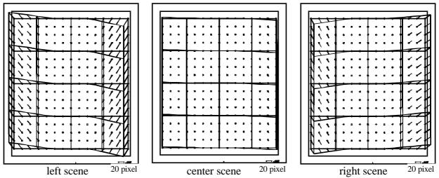
Fig. 5: influence of the special additional parameters for IRS-PAN-images to the scenes
