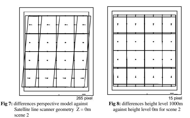
The differences between the satellite line scanner geometry and the perspective model for the center scene of the test data set can be seen in figure 7, it goes up to 265 pixel. These differences
