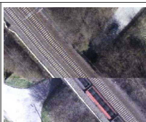
Fig. 11: matching of neighbored orthoimages based on DEMs not including the railway dam
