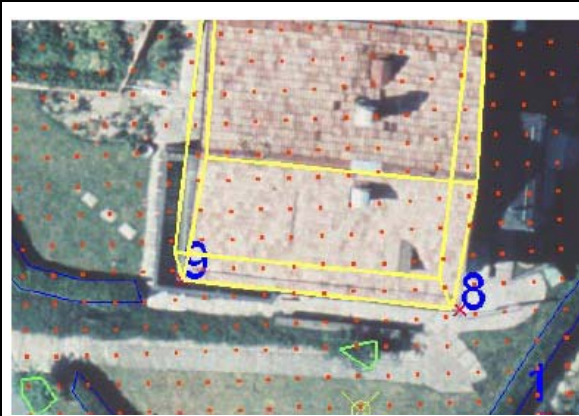
Figure 8: location of a building in a usual orthoimage based on a DEM including the bare ground
