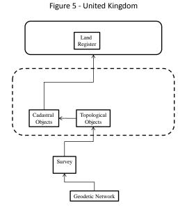
The cadastral fabric is merely a layer of the topographic database, which is generated as "unsharp boundaries" based on the identified and surveyed topographic objects.
