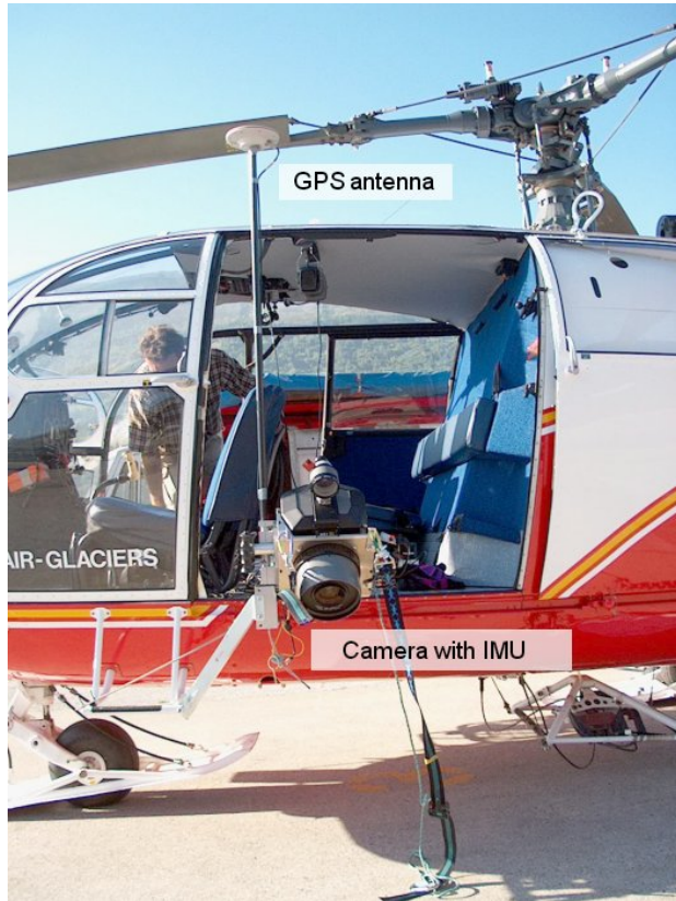
Fig. 3 : Tomtecs camera mounted with GPS antenna. The INS is mounted under the camera. During the picture session, the block camera-antenna is only hold by the operator.
