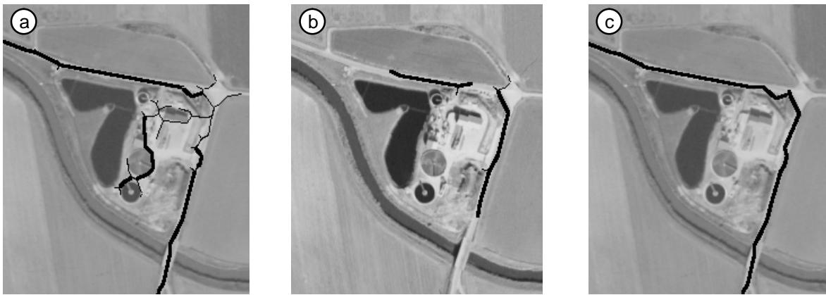
Figure 2. Sensor Fusion demonstrated on the aerial view of a purification plant: Rejected (thin lines) and accepted (wide lines) road features from (a) visual and (b) infrared image with (c) fusion result.
