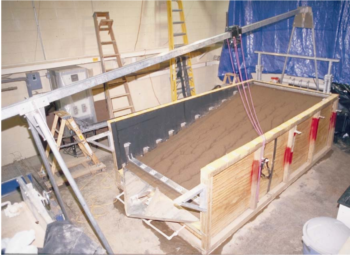
Figure 2. Experimental set up. A 31 % slope was created. Control points have been fixed around the flume. The camera was moved parallel to the soil surface with the apparatus seen above the flume. A rainfall simulator is located further above the flume. Deep and narrow rills formed on the soil surface.
