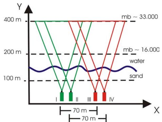
Figure 4. Camera constellation in planimetry
