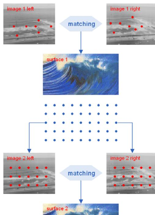
Figure 2. Determination of wave surfaces from image sequences
