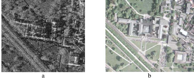
Figure 1. Comparison of SAR and optical image: the main building of the Leibniz Universität Hannover imaged by (a) the TerraSAR-X satellite (© DLR) (high resolution spotlight mode, resolution approx. 1m, range direction left to right) and by (b) an optical aerial sensor (© Geoinformation Stadt Hannover)
