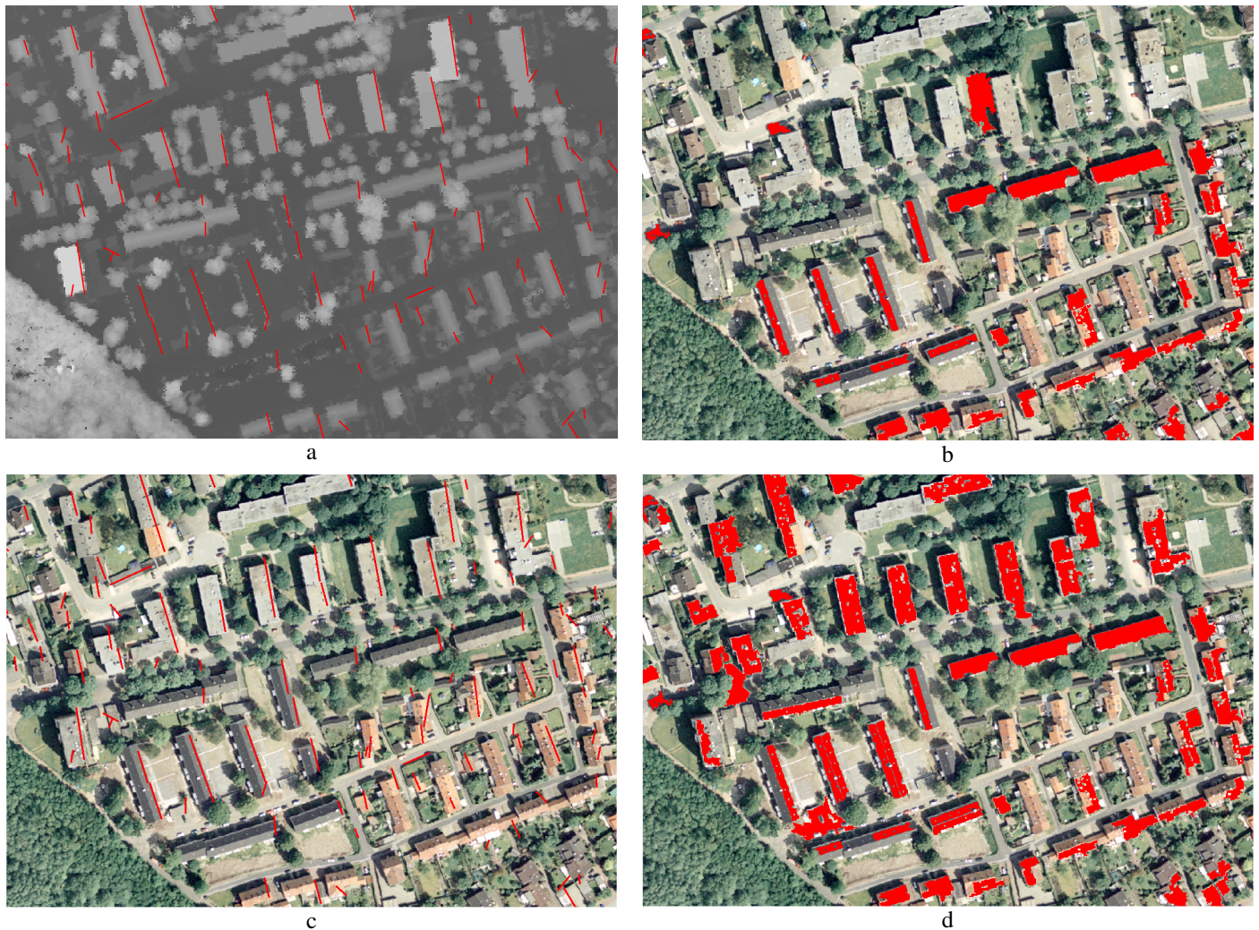
Figure 4 Results of building corner line segmentation based on InSAR data (a, c), of building detection based on optical data (b), and of building detection based on InSAR and optical data (d)
