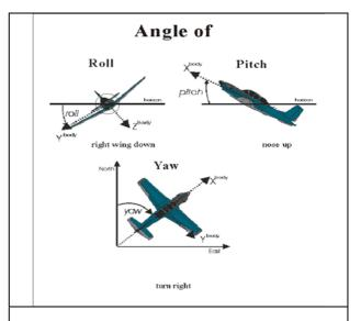
Figure 1: Definition of roll, pitch and Yaw conform to ARINC 705
