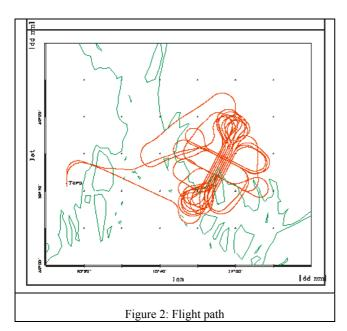
The 1:10000 test flight comprises four parallel strips and one cross strip and covers the whole test field. The cross strip and one of the parallel strips were flown twice in opposite directions, too. Apart from the possibility to check the calibration parameters in another image scale the second scale is required to resolve the high correlation between the vertical GPS shift and the correction of the focal length.
