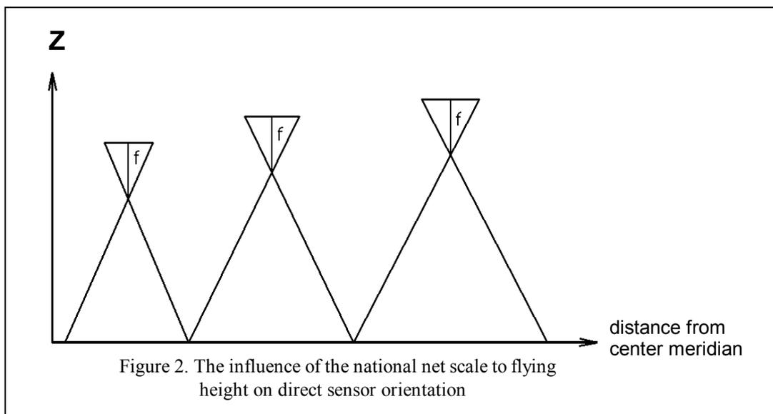
The influence of the affinity model deformation can be compensated for nadir images with a modified focal length with the following relation:  $f_c = f / \text{local scale}$ . This will compensate the difference between the horizontal and vertical scale in a sufficient manner. The used geometric configuration including the individually modified focal length has to be respected for the whole photogrammetric process up to the photogrammetric workstation.
