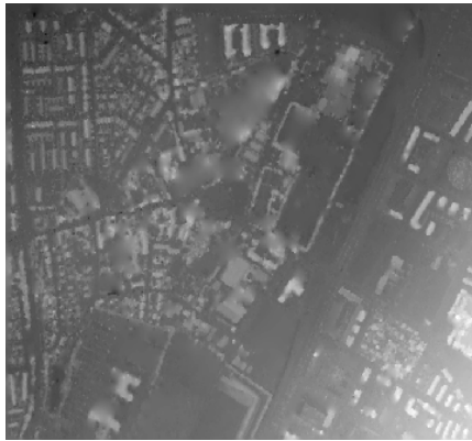
Figure 2. (a). Grey value coded DSM of test area without filtering
