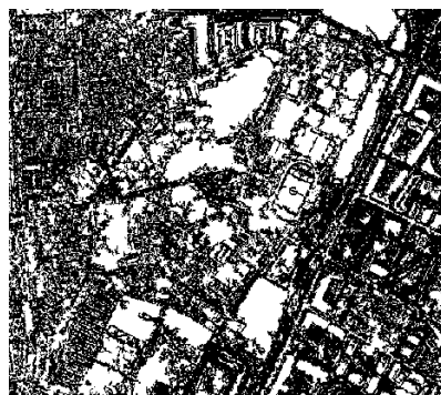
(b) Points determined by automatic image matching
