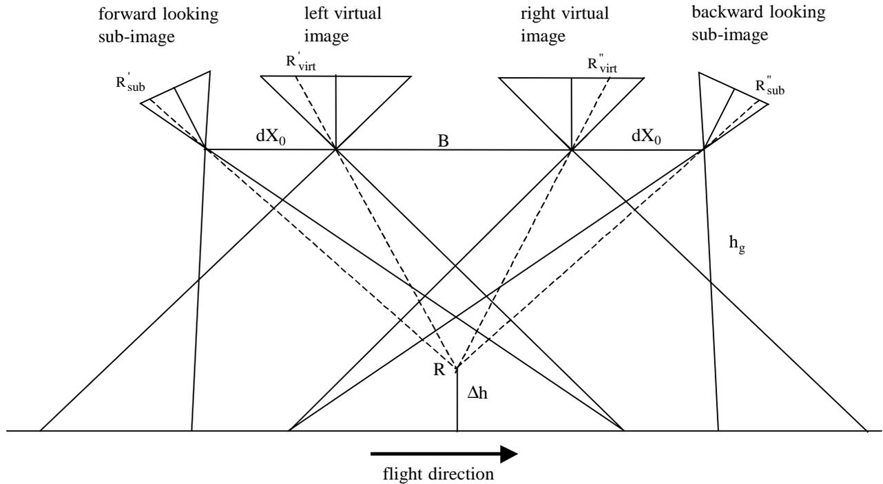
Fig. 4 : DMC stereo model and the height displacement
