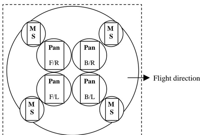
Fig. 1. DMC standard constellation with four panchromatic (Pan) and multi-spectral (MS) modules, where
