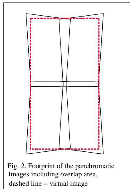
Fig. 2. Footprint of the panchromatic Images including overlap area, dashed line = virtual image
