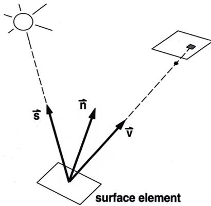
Figure 1: Relationship between direction of illumination  $s$ , surface normal  $n$  and viewing direction  $v$
