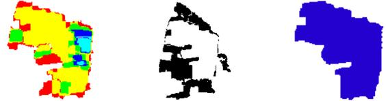
Figure 3. Left: overlap count for the best planar segment (segment B) in Fig. 1. Red / yellow / green / blue / cyan: 1 / 2 / 3 / 4 / 5 overlapping segments. Centre: regions belonging to non-co-planar matching candidates (black). Right: final roof segment.
